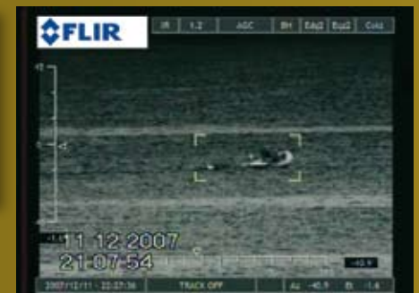
The Vilga video tracking board will allow the camera to follow an object as long as it can be seen.
