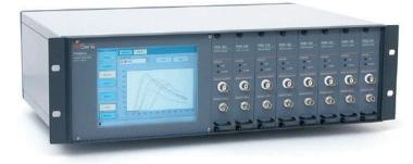
PSC-D RADSENS CHASSIS DEDICATED FOR HIGH SPEED TEMPERATURE MEASUREMENTS
